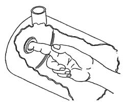
Figure Y Remove Stationary part of seal
